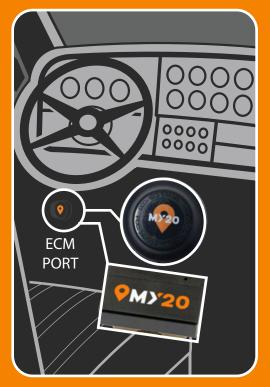
To install the MY20 ELD, match the pin configuration on the back of the ELD to your ECM connector (9pin or OBDII). Once the center pin "key" is aligned in the "slot", push the device to fully seat it, and then turn the outer locking ring clockwise (to the right) by 1/8 of a turn to lock it in place
